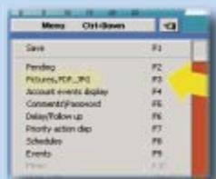
During alarm processing, accounts images can be accessed directly by clicking (F3) or right click and select layouts/pictures. A flashing box in the alarm processing window is another clue to the presence of images in the account file.
